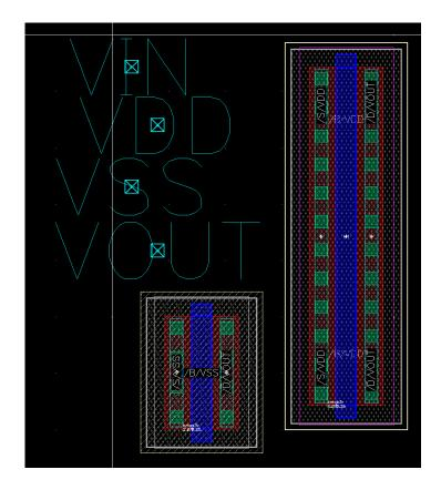
Ensure that all pins have a label, large text, with the name of the pin. These are vital to passing LVS later in the lab. If these are not present, either generate the layout again or place the pins individually using create -> pin.
