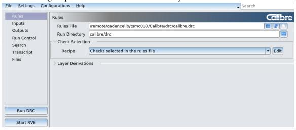
Make sure to run DRC frequently when working on the layout. There are many design rules that are checked by this tool, and fixing them is important.
