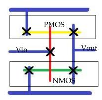
Finish the inverter by adding an n-channel transistor and the necessary connections to make your design look like the stick diagram. You already have the p-channel device so you will need to add the n-channel transistor as well as a Metal 1 line on top for Vdd and one on the bottom for Vss. You will also need to actually connect the drains and sources of the n-channel and p-channel devices with vias and Metal 1, but we will do that in the next few steps.
