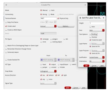
Create the pins for your Input, Output, and  $V_{SS}$  and  $V_{DD}$ . Once complete, run a DRC on your circuit.
